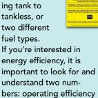
Operating efficiency, sometimes called thermal efficiency, is the percentage of energy that a water heater turns directly into hot water. Any energy loss during operation (when the burner or heating element is on) lowers this percentage. A more important figure is the energy factor: the water heater's average efficiency over a 24-hour period, which incorporates all types of energy loss. This number is expressed as a decimal but translates directly into a percentage for comparison's sake.
